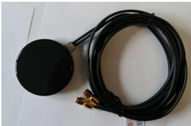
The form of connectors for the GPS/GSM antenna cable are basically identical (SMA form).
