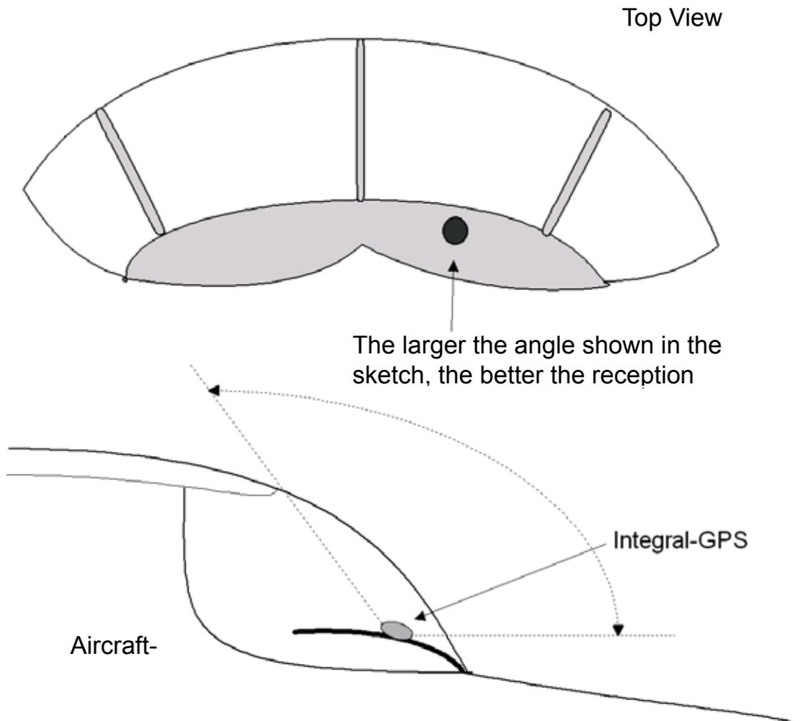
Please consider the shadowing effect of the rotor and possible interference from the ignition box.
