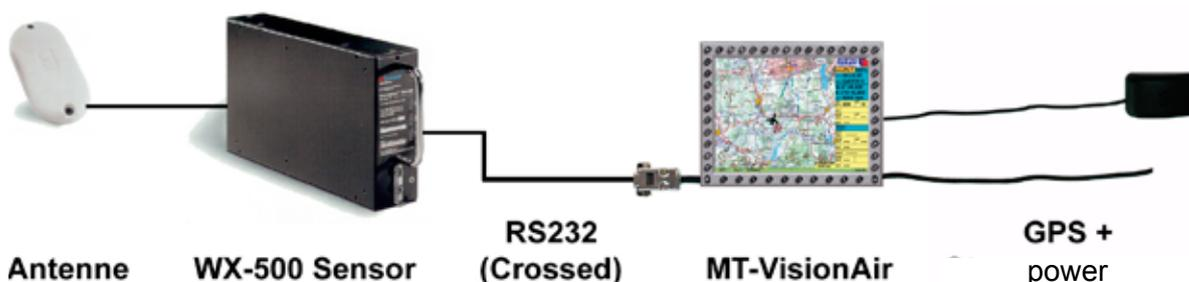
The components of the system must be correctly connected:
