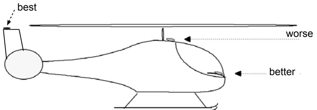
Notice: The integral GPS can also be mounted on the outside of the aircraft. In general a temperature limit of -20°C must be observed.
