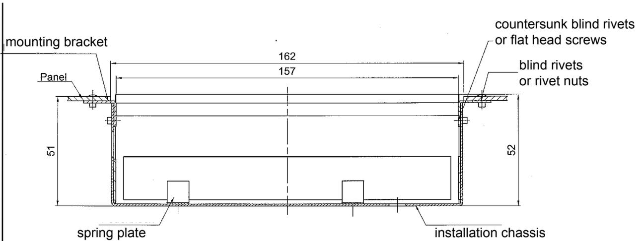
Please use flat head screws for installation in the instrument panel (or onto the angled rail) as space of 158 mm including any protruding screwheads must remain available for the device.
