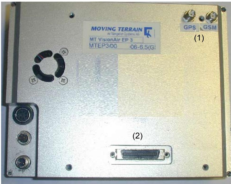
By default a GPS/GSM combination antenna with SMA connectors is attached to this system version:
