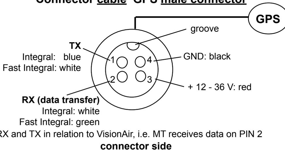
**Important!** Make sure which GPS you are connecting (**Fast Integral GPS** or **Integral GPS**) in order to get the right color code for the cables (see p 22).
