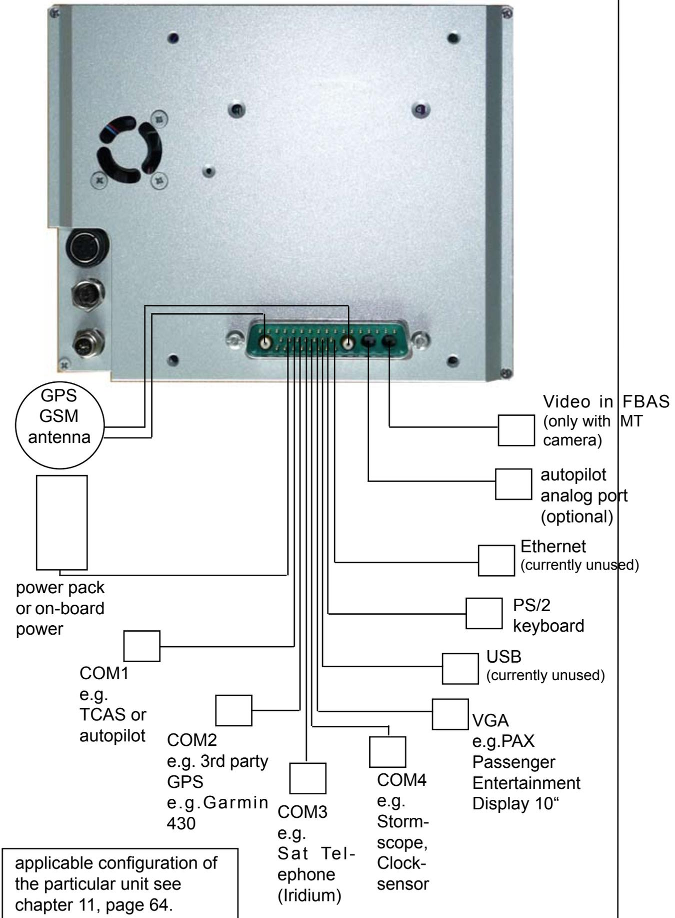
**Pin assignment 36W4 central connector including coax contacts**
