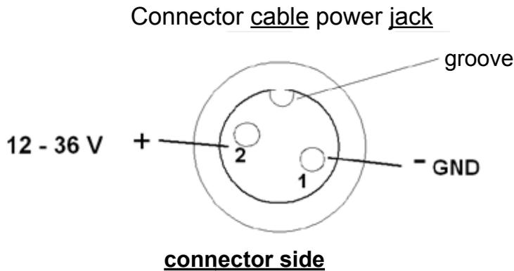
Gnd has to be connected before start-up!!
