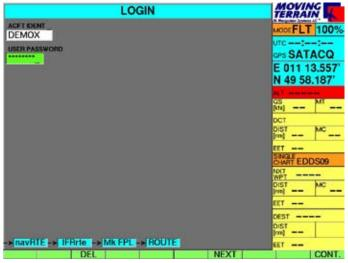
The MT VisionAir login panel has two highlighted input lines. The login panel is normally accessed only once during each program execution. If it is required to return to the login page, the unit must be switched off and restarted.
