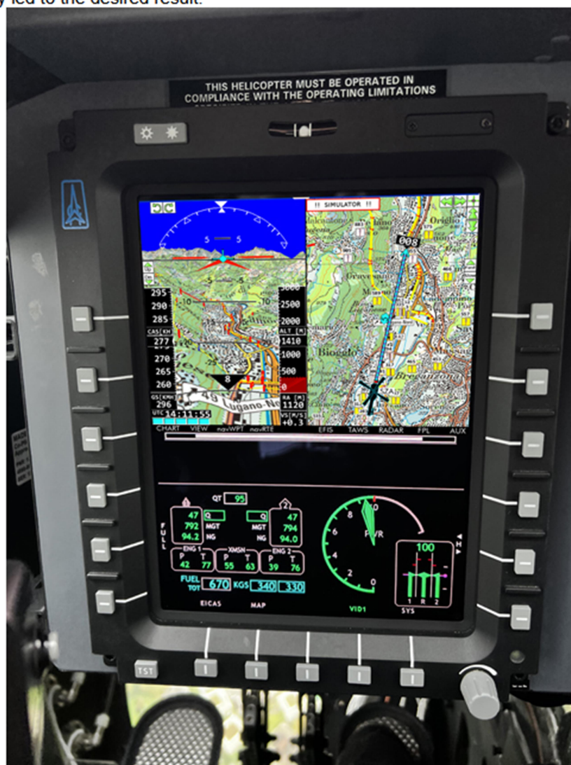
Left DU in detail: Split screen 3D Terrain EFIS and 2D Moving Map + obstacle warning in 2D and 3D
