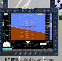
MT Terrain EFIS: display of real time flight attitude
