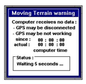
Your GPS is not connected, defective or you have set the wrong COM port. Solution: Check to ensure that your GPS operates independently. Check the COM port setting and cable connections.
