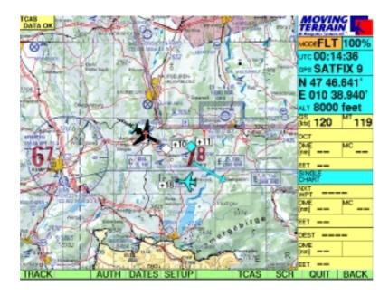
The TCAS mode is shown at the top left of the main window. If DATA OK appears, TCAS data is being received. If NO DATA appears, no TCAS data is being transmitted.
