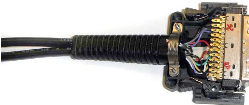
Fig. 5.6.4 (4): Soldered shieldings and connector to device ground
