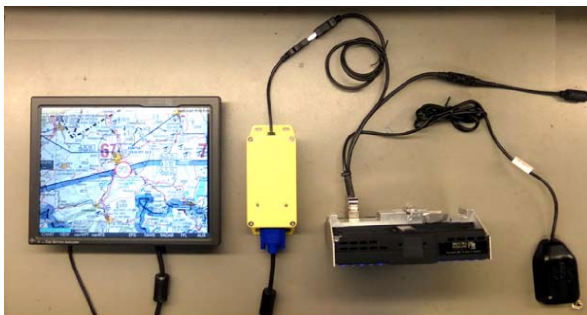
External Screen Power VGA MT-VGA-Output VGA MT-VisionAir X: central connector with USB Power Fast Integral GPS
