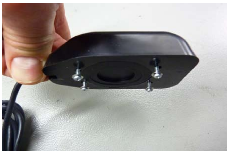
Fig. 4.1.2.(2): Side view of Fast Integral GPS - screws can be used, but we recommend fastening with velcro
