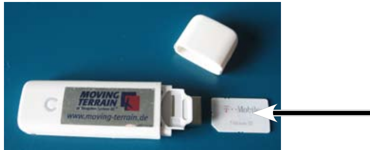
Fig. 9.1.1: SIM-card insertion direction (UMTS-Modem)
