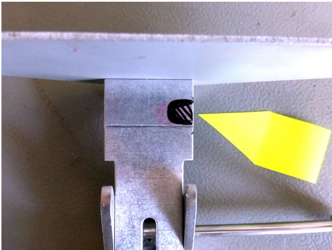
Easy mount with marked notch (front view detail, turned 90° counter clockwise)
