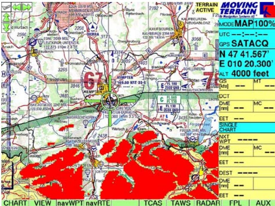
The display consists of a layer on the map with reference to the current (simulated) altitude. Using the keys
