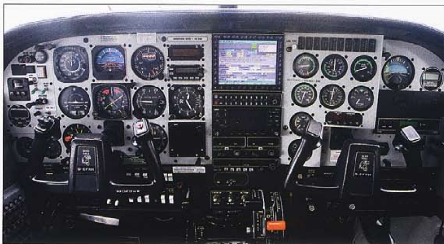
The VisionAir clicks into place in the avionics stack. Updates are easy via a CF card
